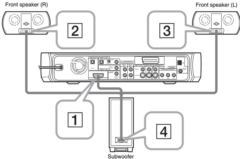
Connect the speaker cord in order of **1** to **4**, according to the above illustration.
