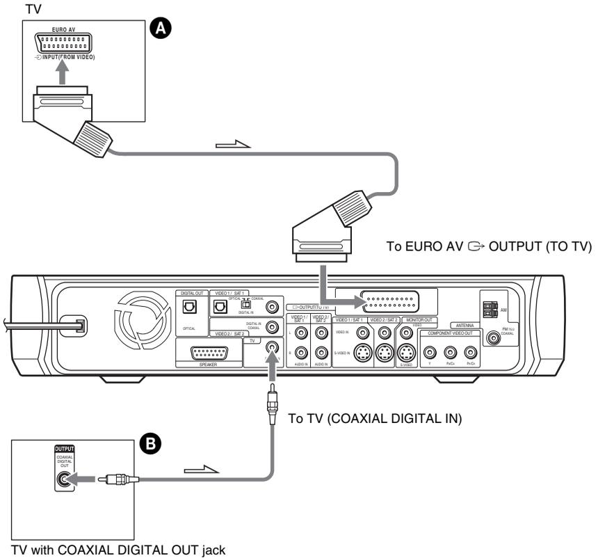
**A To connect the EURO AV INPUT (FROM VIDEO) jack of a TV to the EURO AV OUTPUT (TO TV) jack of this system**
