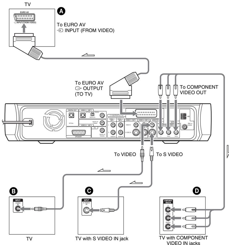
**A To connect to a TV with the SCART input jack**
