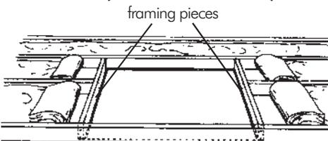
FIGURE 5B (Joist-In Installation)
