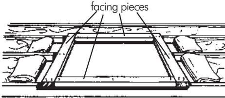
**FIGURE 6B (Joist-In Installation)**
