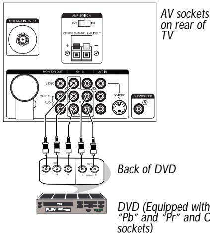
You can view the playback of DVD discs by using the **COMPONENT VIDEO INPUT** sockets on the rear of the TV.
