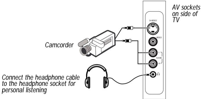
For more convenient direct playback connections, the Side Audio/Video Input sockets allow for quick and easy connections, particularly Camcorder tape recordings.
