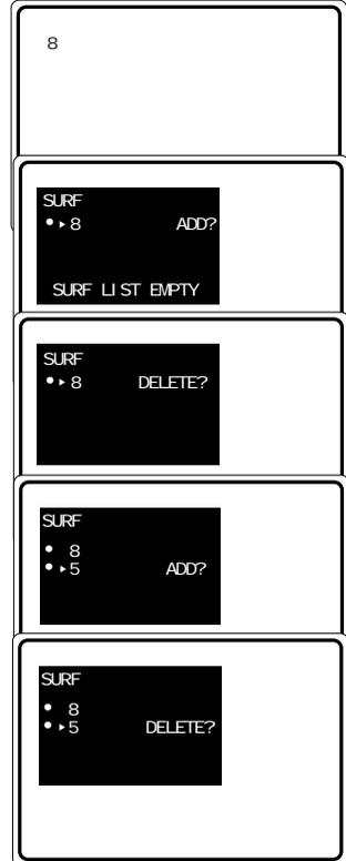
**Note :** To view the the selected channels in the surf list, press the **SURF** button repeatedly to cycle through the channels.
