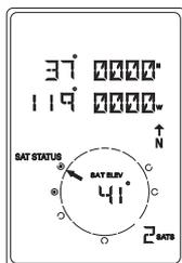
As the GPS 300 searches for satellites, some of the small circles around the large circle will become black indicating that the GPS 300 is tracking that satellite and receiving information. The number at the bottom right of the screen displays how many satellites are being tracked.
