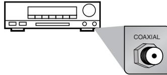
Audio Coaxial Digital cable (commercially available)
