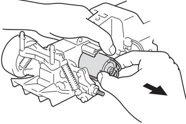
7. Place the new motor so the connectors are vertically aligned, then push the motor all the way in.
