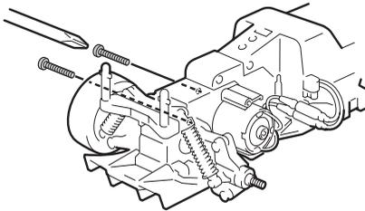
6. Remove the motor from the chassis.
