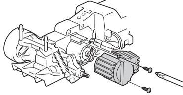
4. Remove the plastic cover from the wires to expose the connectors. Detach the wires by holding the connectors. Do not pull the wires.
