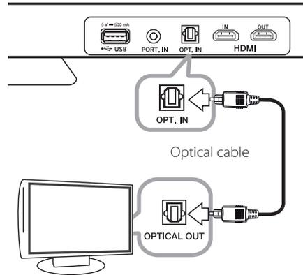
2. Set the INPUT source to OPTICAL. Press repeatedly **FUNCTION** on the remote control or **F** on the unit until the function is selected. For selecting directly the OPTICAL function, press **OPTICAL** on the remote control.
