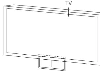
3. When you mount it on a wall (concrete), use the wall plugs. You should drill some holes. A guide sheet (Wall Mount Bracket Installation Template) is supplied to drill. Use the sheet to check the point to drill.
