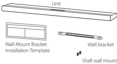
1. Locate the shaft wall mount on the screw hole of the unit's back and then fix it onto the unit with the screw.
