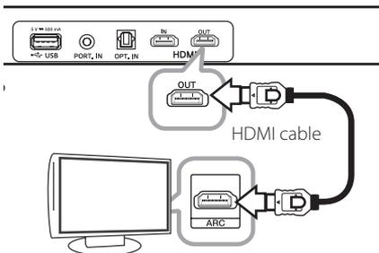
2. Turn TV and the unit on. ARC function is selected automatically.
