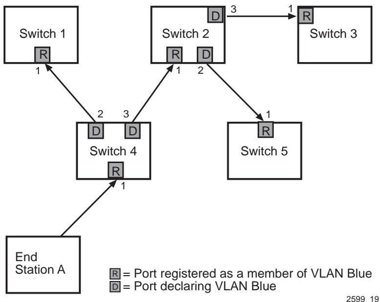
**Figure 4-1** Example of VLAN Propagation via GVRP
