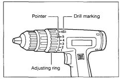
Before actual operation, drive a trial screw into your material or a piece of duplicate material to determine which torque level is required for a particular application.
