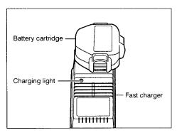
minute. Then re-insert it and try to charge it once more. If the charging light goes out within one minute even after repeating this procedure a couple of times, the battery cartridge is dead. Replace it with a new one.
