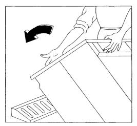
Remove the polystyrene panel from underneath the machine.
