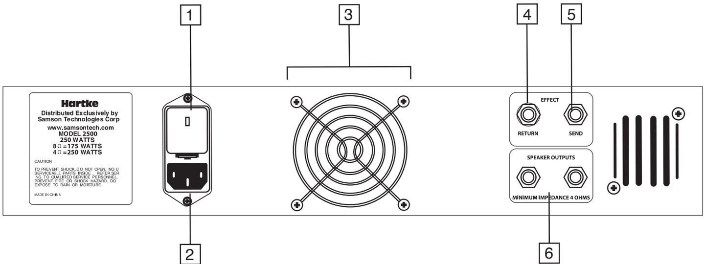
**1. Fuse sled** - This contains a fuse holder and shows the currently selected voltage rating for your Model 2500. Make sure the voltage rating is correctly set before powering up the amplifier! Fuse ratings are 10 amp for 115 vac and 6.2 amp for 230 vac. For information on how to change the voltage rating, see Appendix B on page 14.
