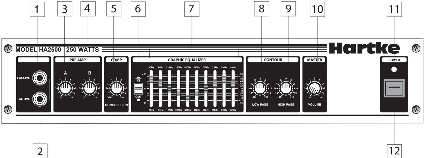
**1. Passive Input jack** - If your bass guitar has passive circuitry, connect it to the Model 2500 here. This standard, 1/4" unbalanced jack provides a high impedance (100 k Ohms) input sensitivity of 20 millivolts.
