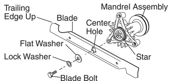
If bolt needs replacing, replace only with approved bolt shown in the Repair Parts.
