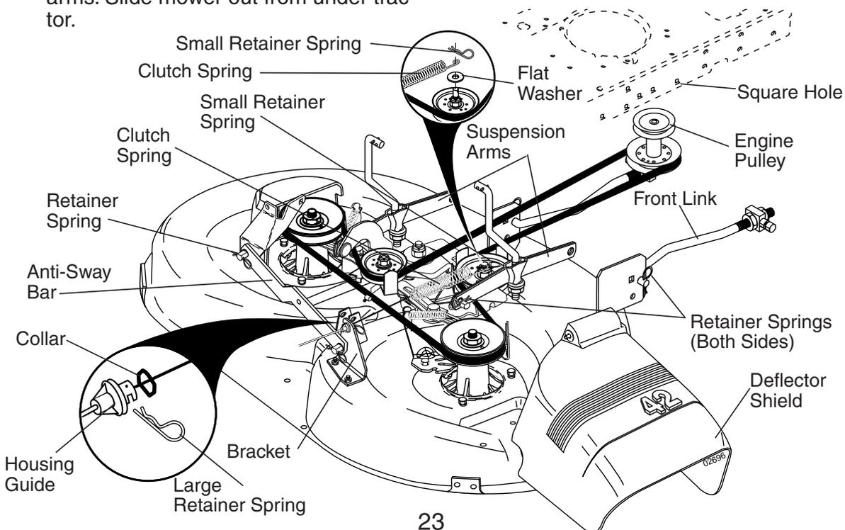
8. Place flat washer and clutch spring on idler pulley bolt and secure with small retainer spring.
