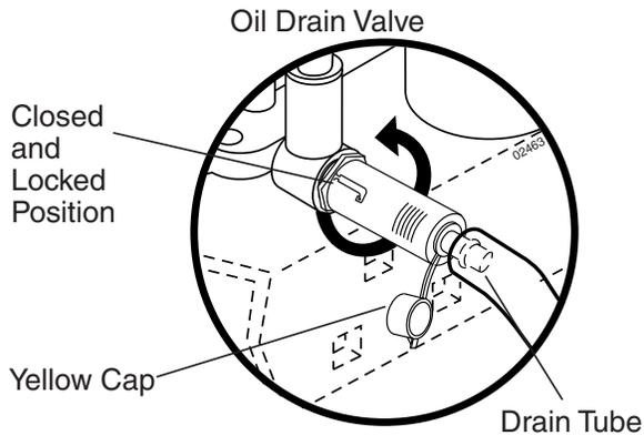
3. Unlock drain valve by pushing inward slightly and turning counterclockwise.
