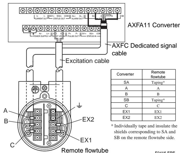
Figure 4.4.6 Wiring Diagram
