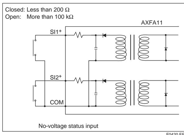
Figure 4.4.12 Status Input Connection
