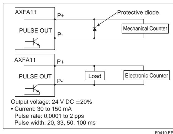
Figure 4.4.11 Active Pulse Output (Optional code EM)
