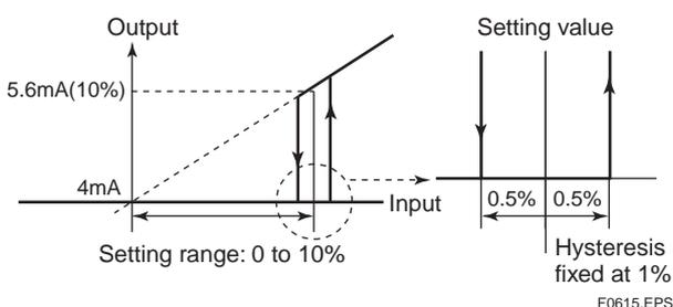
**[J11: 4-20mA Low Lmt]** Setting of the low limit for current output
