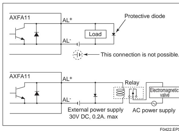
Figure 4.4.14 Alarm Output Connection
