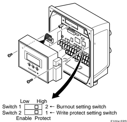
Figure 10.1.4 Switch Configuration
