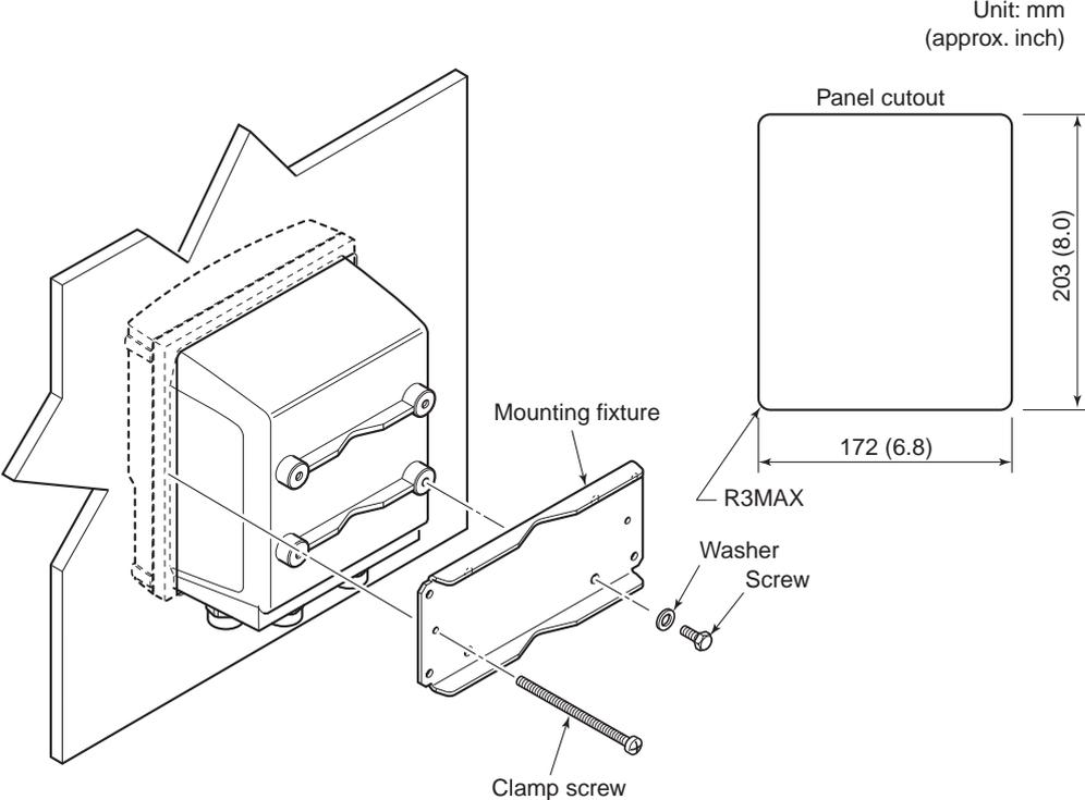
Fit the AXFA11 into the panel. Then attach the mounting fixture to the AXFA11 using the screw and the washer, and secure the instrument with the two clamp screws.
