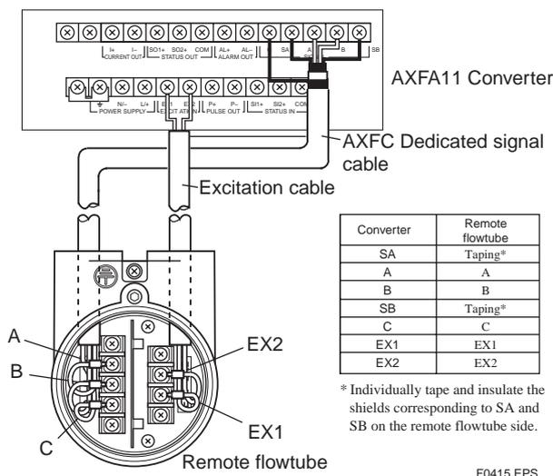
Figure 4.4.5 Wiring Diagram
