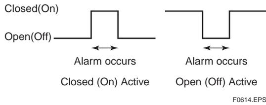
**[G21: 4-20mA Alarm Out]** Setting of the current output during an alarm occurrence
