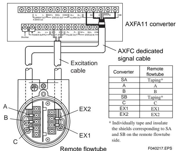
Figure 4.4.7 Wiring Diagram
