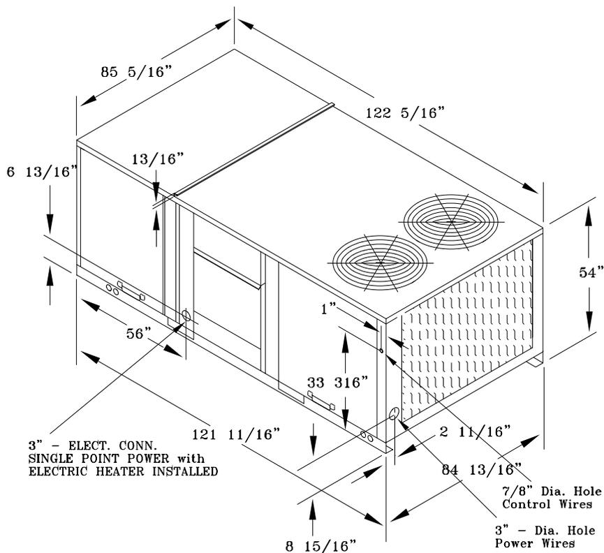
**Figure 5. Roofcurb Dimensional Data 20 Ton**
