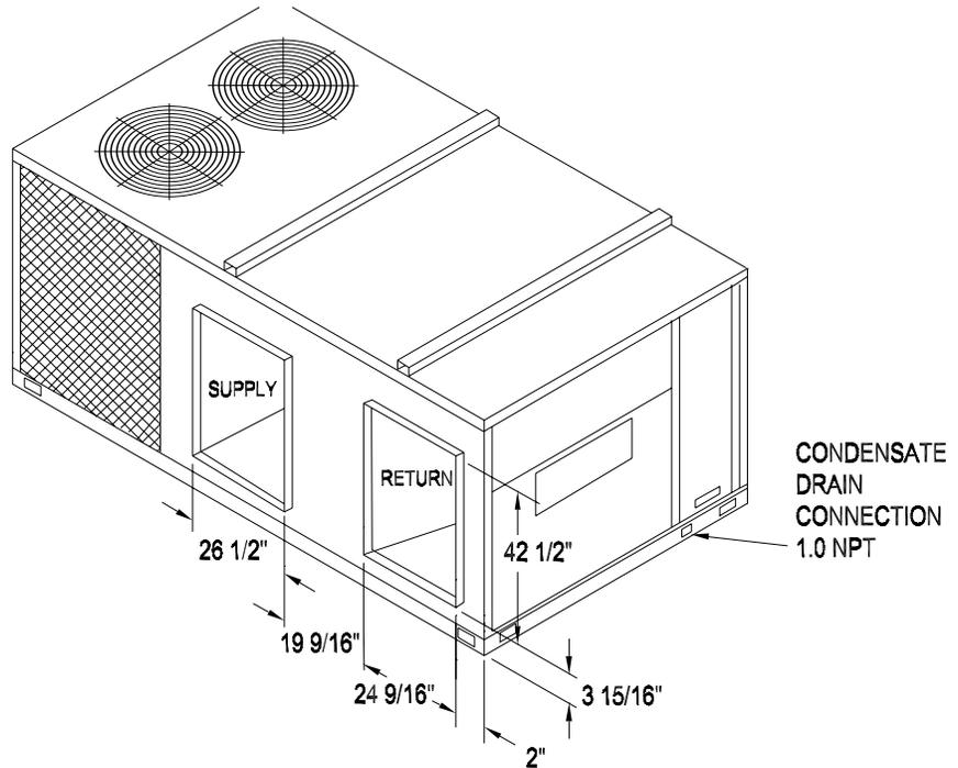
Figure 7. Horizontal Duct Dimensional Data 20 Ton
