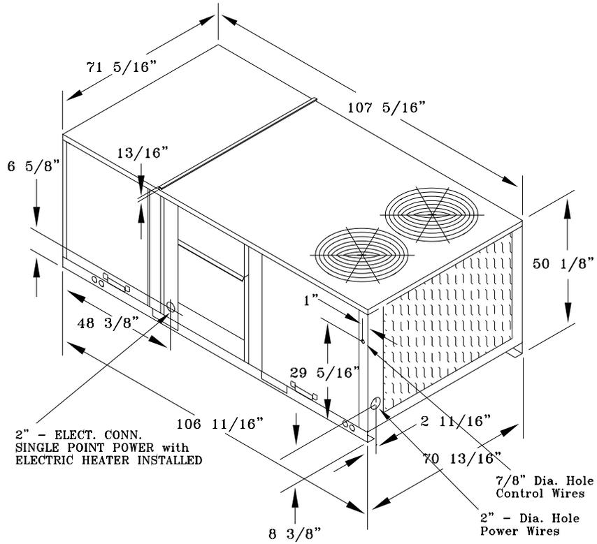
**Figure 3. Roof Curb Dimensional Data 12 1/2 Ton, 15 Ton**
