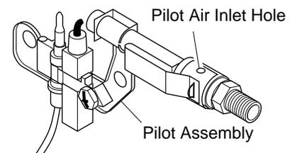
Figure 21 - Pilot Inlet Air Hole
