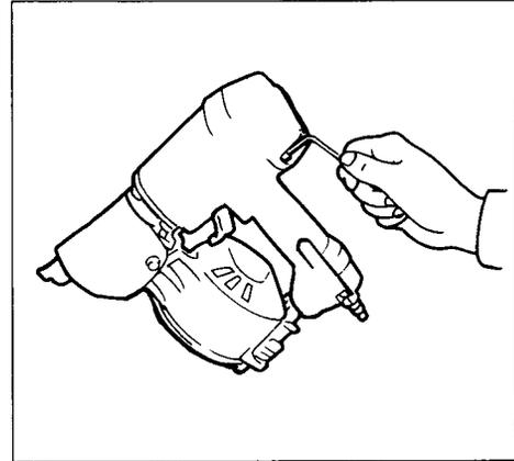
Make sure all safety systems are in working order before operation. The tool must not operate if only the trigger is pulled or if only the contact element is pressed against the wood. It must work only when both actions are performed. Test for possible faulty operation with nails unloaded.
