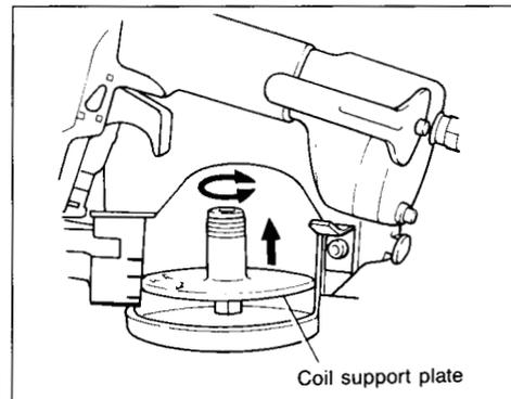
Place the nail coil over the coil support plate. Uncoil enough nails to reach the feed claw. Place the first nail in the driver channel and the second nail in the feed claw. The nail heads must be in the slot in the feeder body. Place other uncoiled nails on feeder body. Close the magazine cap and door after checking to see that the nail coil is set properly in the magazine.
