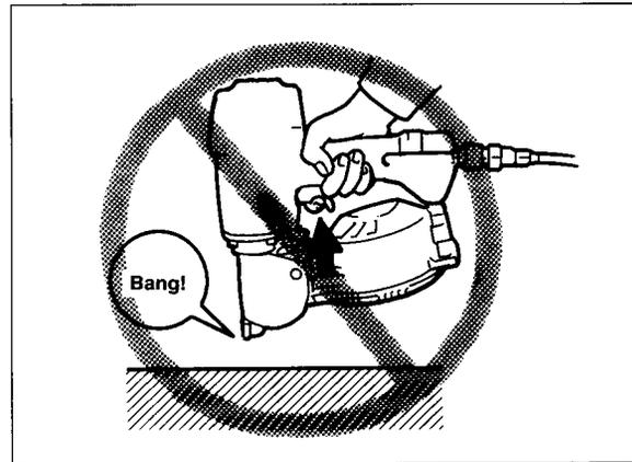
Make sure that the trigger is locked when the change lever is set to the LOCK position.
