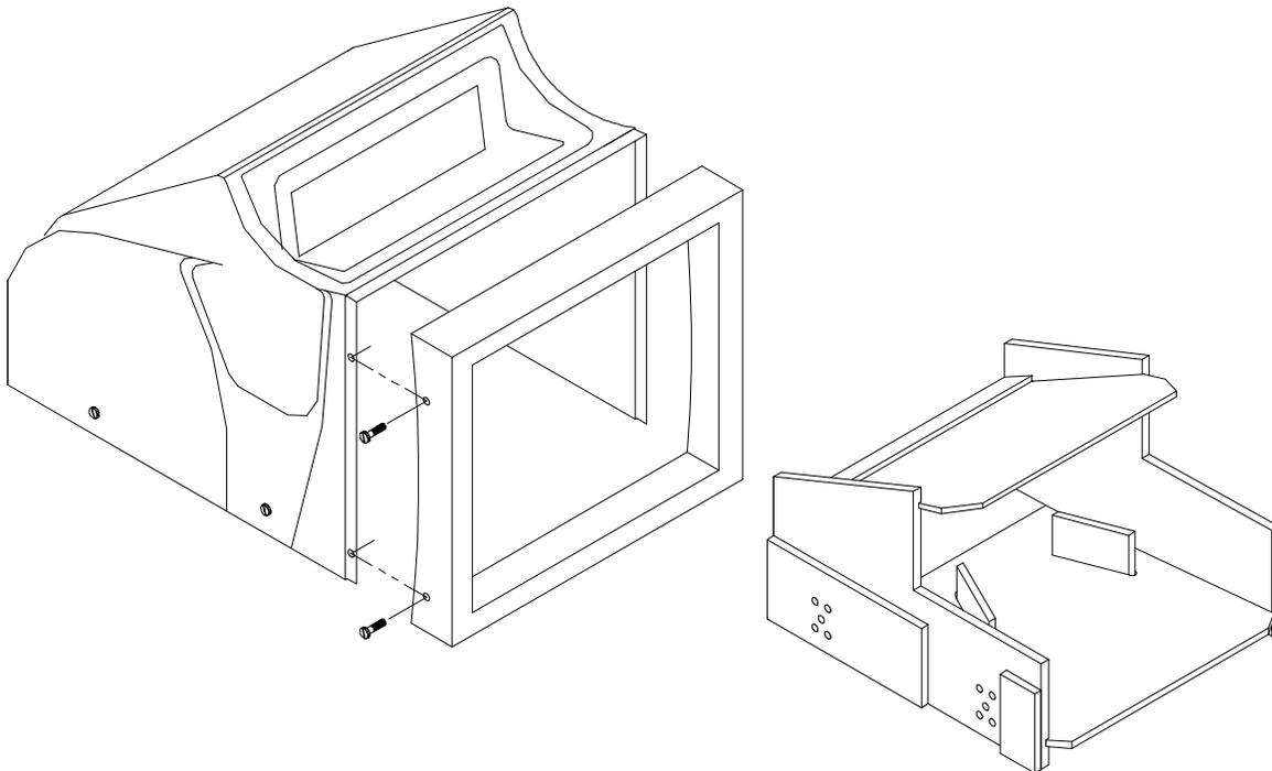
3) Pre-drill pilot holes on side of VCP shelf (A) and on bottom of TV shelf (B) using 1/8" drill bit.
