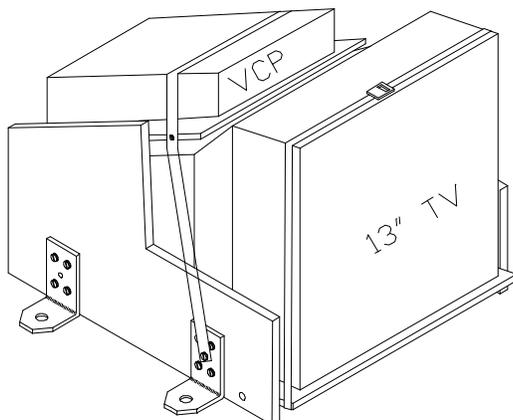
**Step 6) Replace the rear shroud and face of console.**
