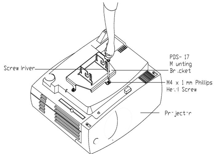
1. Invert the projector and place it on a soft and flat surface. Remove any foot levelers that might possibly prevent the correct installation of the bracket.
