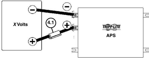
See Battery Connection, Pg.8. 4.1 is the fuse. X = Your APS's Inverter's Nominal Input Voltage. (See specs.)
