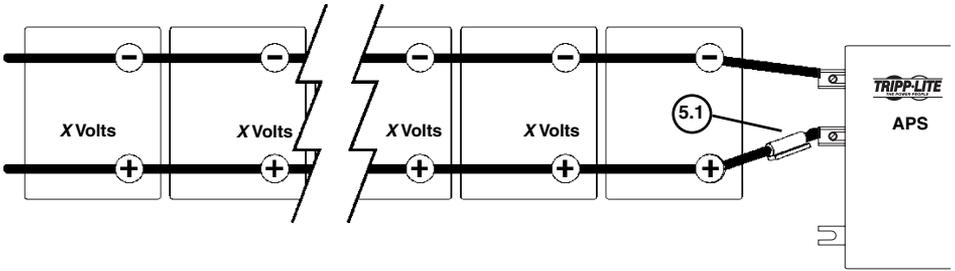
See Battery Connection, Pg.8. 5.1 is the fuse. X = Your APS's Inverter's Nominal Input Voltage. (See specs.)
