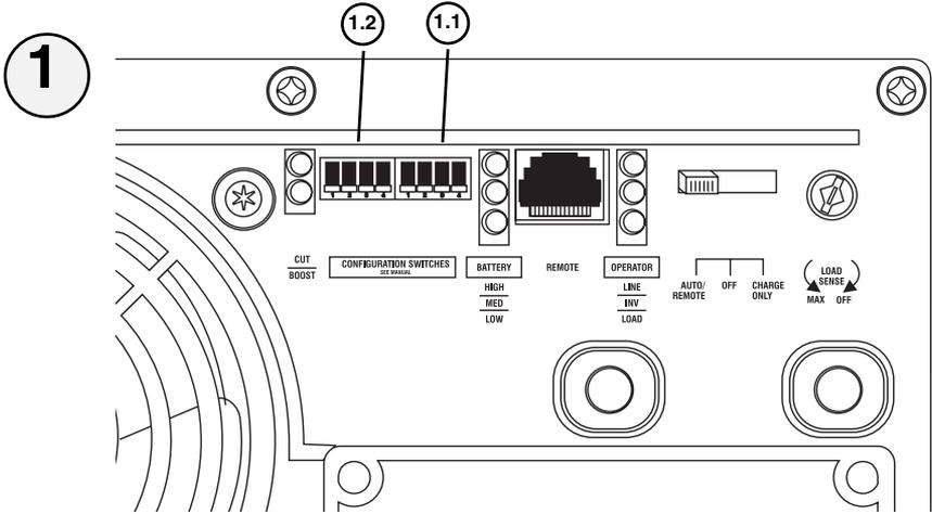
See "Configuration", pg. 5. 1.1 is DIP Switch Group A. 1.2 is DIP Switch Group B.
