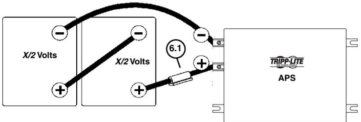
See Battery Connection, Pg.8. 6.1 is the fuse. X = Your APS's Inverter's Nominal Input Voltage. (See specs.)
