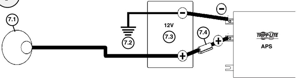
Basic 12VDC Vehicular Battery Connection. See Pg.8.
