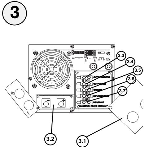
See **Hardwire Electrical Connections**, pg. 9. 3.1 is the cover plate, 3.2 is the five-position terminal strip, 3.3 is the output neutral (white), 3.4 is the output hot (black), 3.5 is the ground (green), 3.6 is the input neutral (blue) and 3.7 is the input hot (brown).
