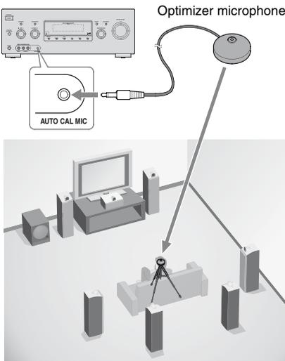
**1** Connect the supplied optimizer microphone to the AUTO CAL MIC jack.
