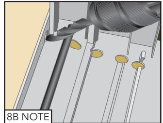
**Note: Ensure that all new or existing weep holes are open before proceeding with the installation.**
