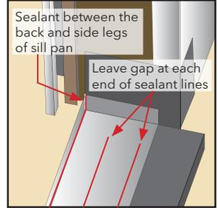
Also seal the joint between the back and side legs of the sill pan with sealant.
