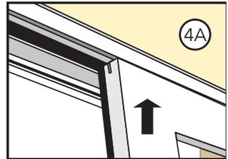
**Note: Make sure the top of the panel clears the anti-lift clip before attempting to place the panel on the bottom track.**
