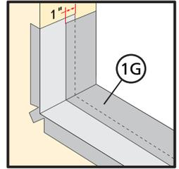
If using optional sill pan, see Step 10 Sill Pan Fabrication and Installation on page 15.
