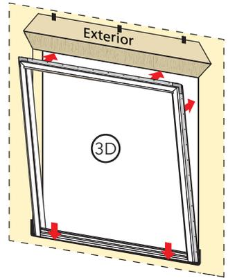
E. **Plumb and square the door.** Insert shims at the jambs between the door and the sides of the rough opening. Place shims behind each of the pre-drilled installation holes. **DO NOT** place shims at the sill. **DO NOT** place shims at the head until Step 4I.
