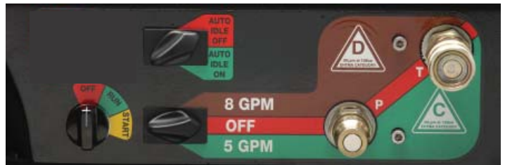
Figure 1. Panel Control Valve
