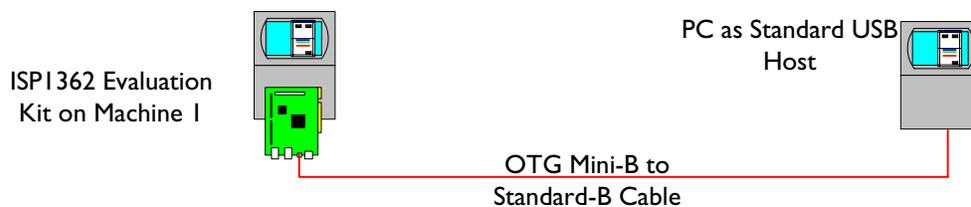
**Figure 4-2: Device Stack Evaluation Setup**
