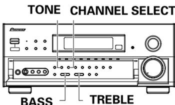
**1 Press the TONE button on the remote control's Amplifier or front panel to put the amplifier in tone adjust mode.**
