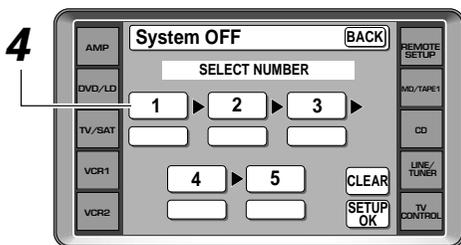
**4 Next you should select the command number you want the process to start with. Of course it's logical to start with 1 so press command 1 button (the box the 1 with inside it).**
