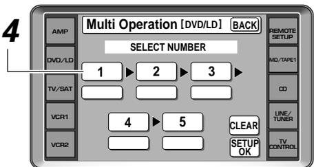
**4 Next you should select the command number you want the process to start with. Of course it's logical to start with 1 so press command 1 (the box the 1 with inside it).**
