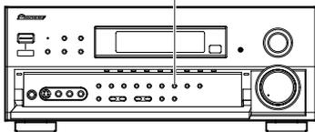
Use the **FL DIMMER** button on the remote control's **Amplifier SUB** screen or the front panel to alternate between the different levels of brightness.
