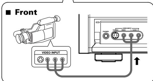
Front video connections are accessed via the front panel input selector as "VIDEO."
