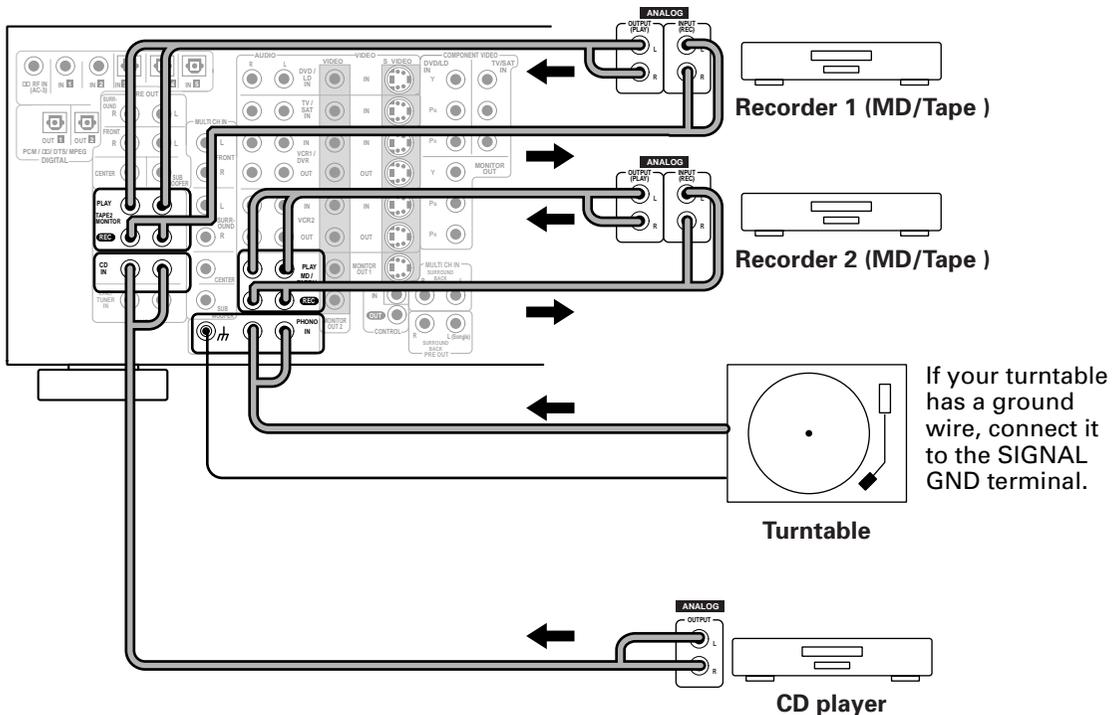
Please don't hook up any other component to the phono jacks other than a turntable. It could damage the equipment. If your turntable has a built-in amplifier please hook it up to the LINE IN or another input other than the PHONO.
