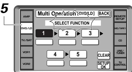
**5 Select the component whose command you want to input (for example, a DVD player), and press that button on the remote control. The LCD screen for that component will appear on the remote control.**
