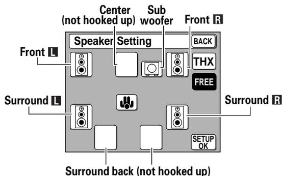
If you don't have a center speaker press the **CENTER** button until the box appears empty. Then press the **SETUP OK** button to **EXIT** and go back to the System Setup screen.
