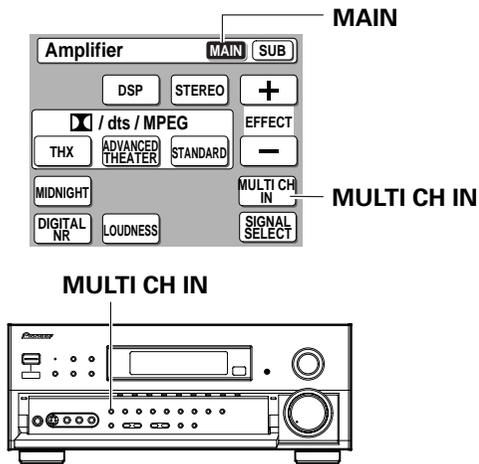
**Press the MULTI CH IN button on the remote control's Amplifier MAIN screen or the MULTI CH INPUT button on the front panel.**
