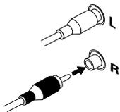
Connect red plugs to R (right) and white plugs to L (left). Be sure to insert completely.
