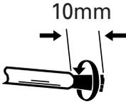
② Loosen speaker terminal and insert exposed wire.
