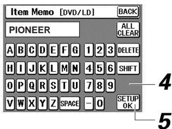
**5 Press the SETUP OK button when the name appears in the bar as you want it on the function screen.**
