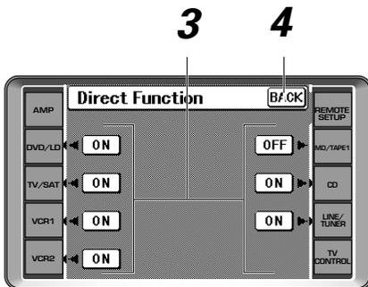
Subsequently the nub will not appear on any remote control screen if the DIRECT FUNCTION is OFF.
