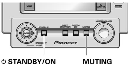
**Hold down both the STANDBY/ON button and MUTING button and then push the RESET tab under the battery cover on the back of the remote control.**
