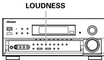
**Press the LOUDNESS button on the remote control's Amplifier MAIN screen or on the front panel.**
