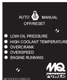
During **cranking cycle**, The MPEC will attempt to crank the engine for 10 seconds before disengaging. If the engine does not engage (start) by the third attempt, the engine will be shutdown by the engine controller's **Over Crank Protection** mode. If the engine engages at a speed (RPM's) that is not safe, the controller will shutdown the engine by initializing the **Over Speed Protection** mode.
