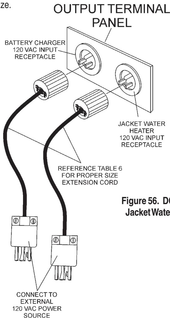
**Figure 56. DCA-45SIU2 Battery Charger & Jacket Water Heater Power Connections**
