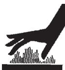
Engine components can generate extreme heat. To prevent burns, **DO NOT** touch these areas while the engine is running or immediately after operations. **NEVER** operate the engine with heat shields or heat guards removed.
