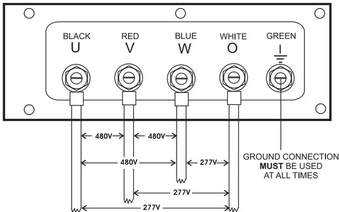
**Figure 28. UVW Terminal Lugs 480/277V Three Phase Connections**
