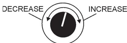
**Figure 24. Voltage Regulator Knob (139V/240V)**
