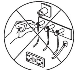
Backfeed to a utility system can cause **electrocution** and or property damage. **DO NOT** connect to any building's electrical system except through an approved device or after building main switch is opened. **ALWAYS** have a licensed electrician perform the installation
