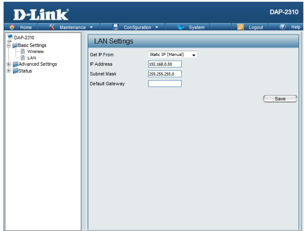
The screenshot displays the D-Link DAP-2310 web interface. The top navigation bar includes 'Home', 'Maintenance', 'Configuration', 'System', 'Logout', and 'Help'. The left sidebar shows a tree view with 'DAP-2310' expanded, containing 'Basic Settings', 'Wireless', 'LAN', 'Advanced Settings', and 'Status'. The main content area is titled 'LAN Settings' and contains the following fields:
