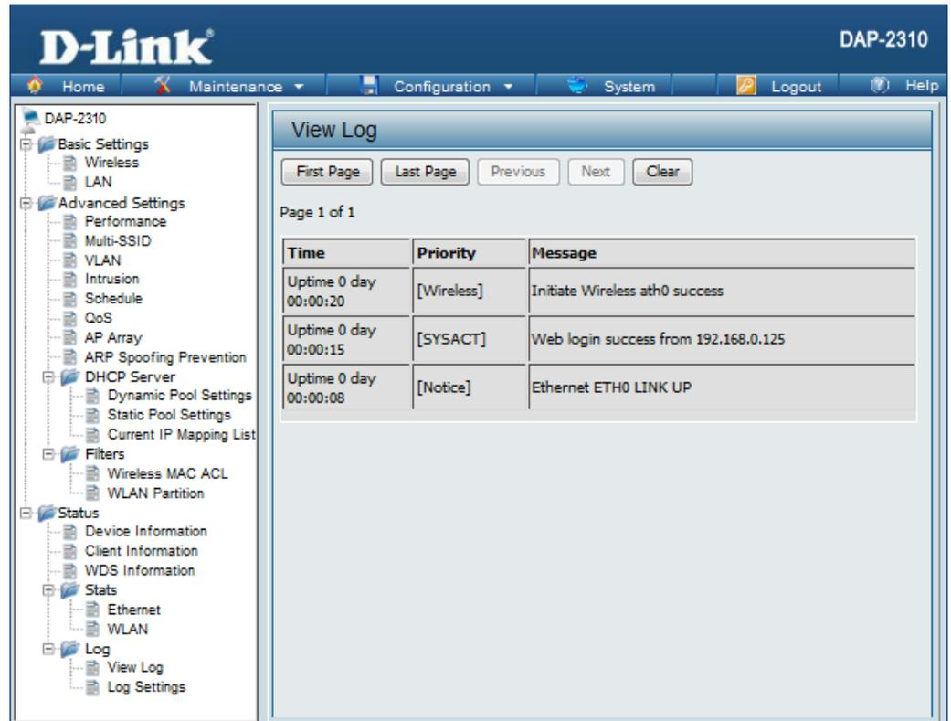
The screenshot shows the D-Link DAP-2310 web interface. The top navigation bar includes Home, Maintenance, Configuration, System, Logout, and Help. The left sidebar menu is expanded to show the Log section, with View Log selected. The main content area displays the View Log page, which includes navigation buttons (First Page, Last Page, Previous, Next, Clear) and a table of log entries.
