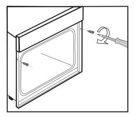
■ Secure the appliance to the left and right side of the cabinet with the two supplied 1/8" x 1" (3.5 x 25 mm) wood screws.
