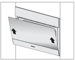
■ Holding the door evenly with both hands, lift the door up at a slant and off the hinges.
