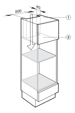
To ensure that the Combi Steam Oven has adequate ventilation, the following cut-outs measuring 19 11/16" x 1 9/16" (500 x 40 mm) must be made:
