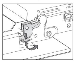
■ Unlock the release levers on both door hinges by pushing on them. Turn the release levers until they click and are in a slanted position.
