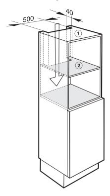
To ensure that the Combi Steam Oven has adequate ventilation, the following cut-outs measuring 19 11/16" x 1 9/16" (500 x 40 mm) must be made:
