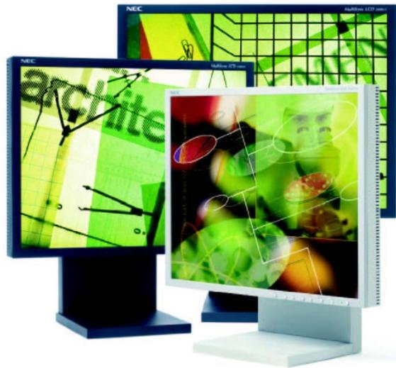
Unlike analog CRT monitors, flat-panel displays and computer projectors are digital devices and are best used with digital (DVI) connections.
