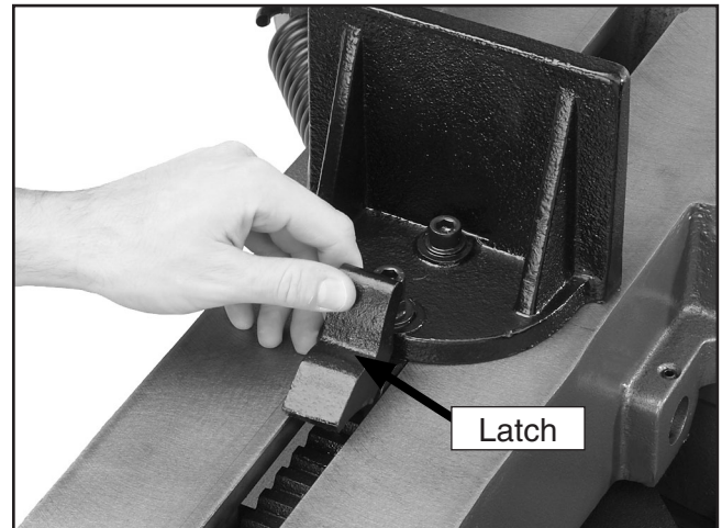
Figure 17. Vise jaw positioning.
