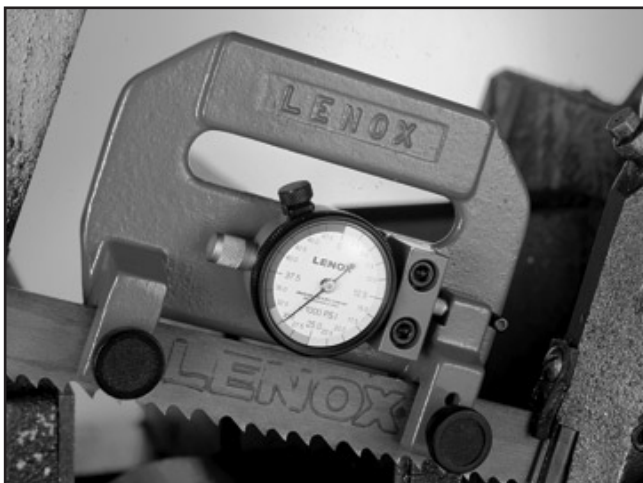
Figure 31. H5408 Blade Tensioning Gauge.
