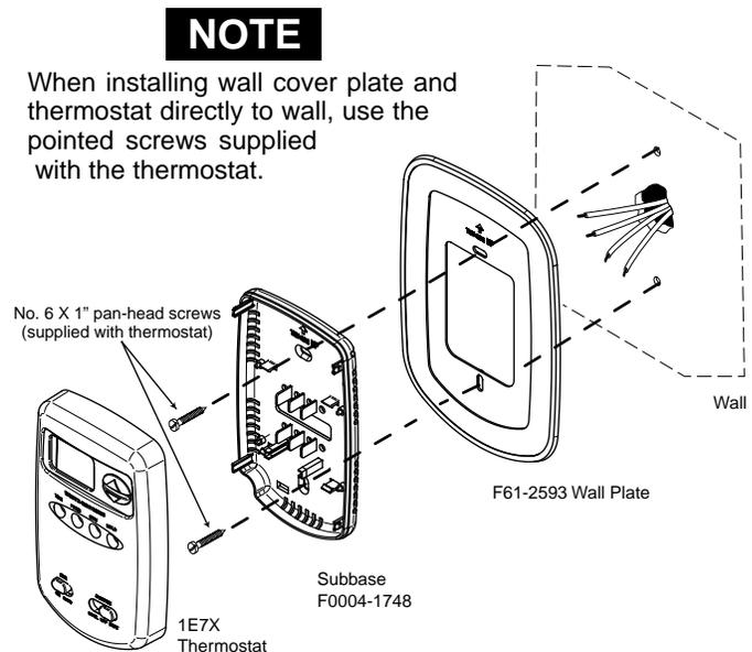
Figure 2. Mounting 1E7X vertical digital thermostat to wall.
