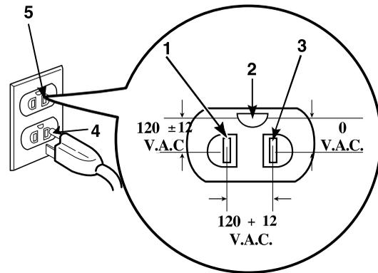
**STANDARD 120 VOLT, 60 HERTZ, 3-WIRE EFFECTIVELY GROUNDED CIRCUIT**
