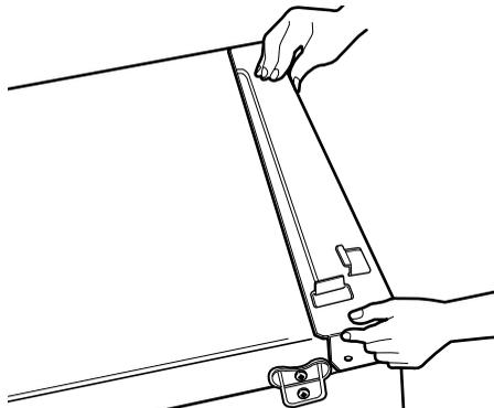
**4** Secure stacking kit side bracket to the washer with a screw on the back of bracket. Repeat Steps 2, 3, 4 for the other side.
