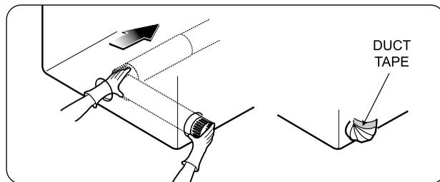
3-2. Insert elbow duct assembly first through the side opening and connect the elbow to the internal duct.
