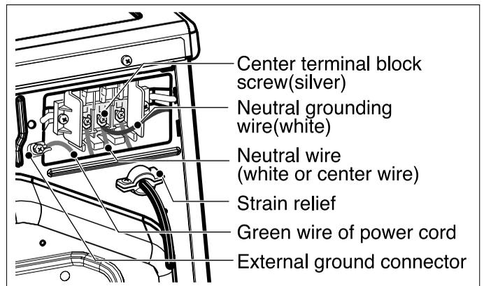
1. Connect neutral wire(white) of power cord to center terminal block screw.
