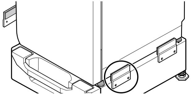
**5** Be sure to press the adhesive parts of the brackets firmly to the appliance.
