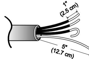
Then, put the hooked shape end of the wire under the screw of the terminal block(hooked end facing rightward) and pinch the hook together and screw tightly.
