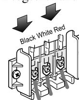
1. Connect neutral wire(white) of power cord to center terminal block screw.
