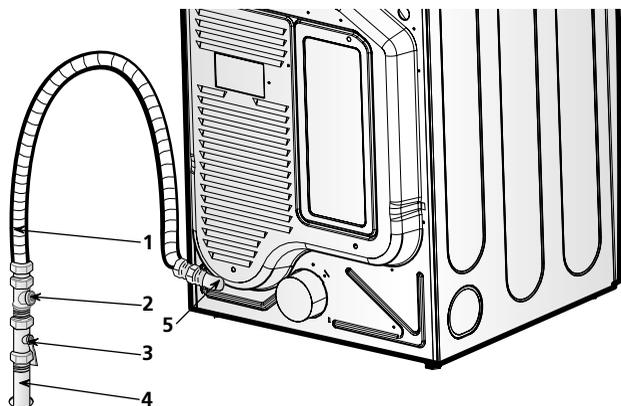
1. New stainless steel flexible connector. Use this type of connector only if allowed by local codes. Use Design AGA Certified Connector.
