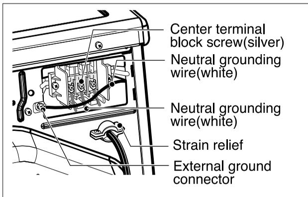
**Option 1: 4-wire connection with a Power supply cord.**
