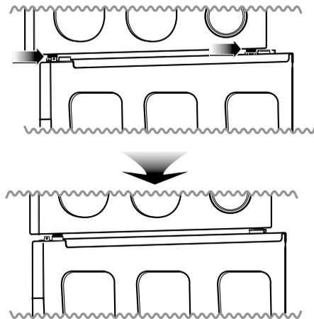
**6** Insert the front stacking kit. Push the front stacking kit back to the stoppers of side stacking kit.
