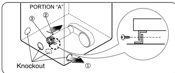
2-2. Reconnect the another duct[11 in(28cm)] to the blower housing, and attach the duct to the base. (Duct is a SVC part)
