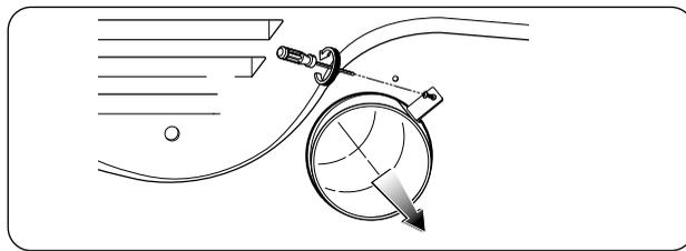
2-1. Detach and remove a knockout at the button, left or right side as desired. (Right Side Vent not available on Gas dryer)
