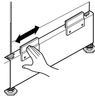
**6** Install the eight (8) screws(supplied) to attach the brackets to the pedestal.
