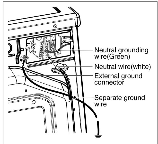
1. Connect neutral wire(white) of power cord to center terminal block screw.
