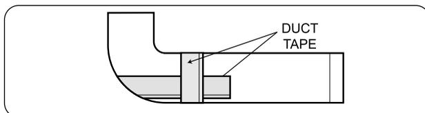
3-1. Pre-assemble 4" elbow with 4" duct. Wrap duct tape around joint.
