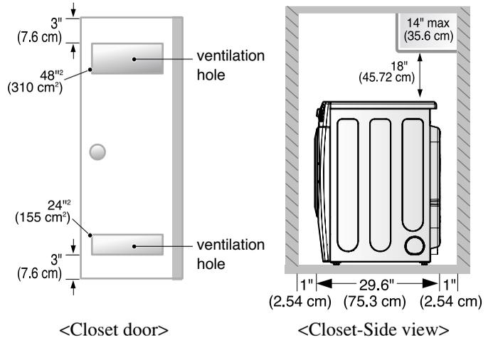
\* Most installations require a minimum 5 1/2 in. (14 cm) clearance behind the dryer for the exhaust vent with elbow.
