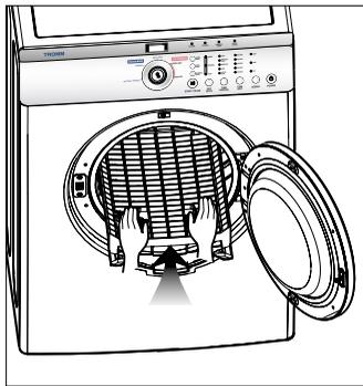
**3. Make sure that dryer is evenly placed right onto the drum inside and door rim.**
