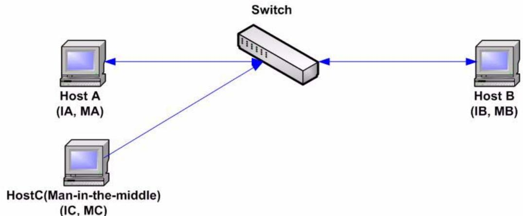
Hosts A, B, and C are connected to the switch on interfaces A, B and C, all of which are on the same subnet. Their IP, MAC addresses are shown in parentheses; for example, Host A uses IP address IA and MAC address MA. When Host A needs to communicate with Host B at the IP layer, it broadcasts an ARP request for the MAC address associated with IP address IB. Host B responds with an ARP reply. The switch and Host A update their ARP cache with the MAC and IP of Host B.
