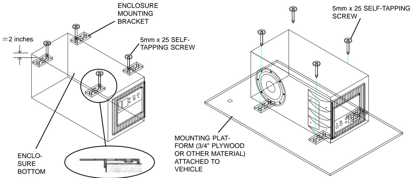
2. Attach each bracket using four of the 5mm x 25 self-tapping screws supplied.
