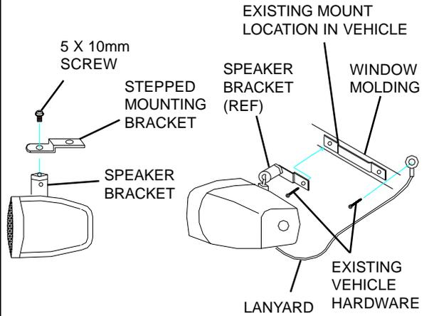
**2. Mounting the Speaker over the Rear Molding:**
