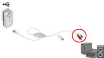
Or, use the 3.5 mm mini jack to connect a speaker with the mini jack connector.
