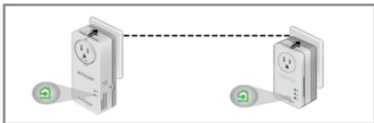
3. On each adapter, press the **Security** button for 2 seconds and then release.
