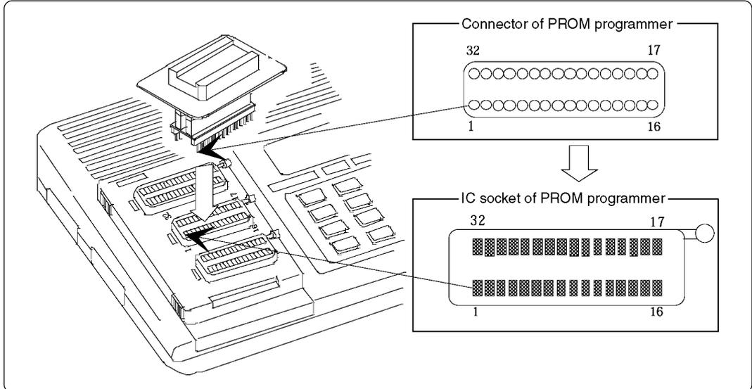
Figure 3.1 Attaching the adapter to a PROM programmer
