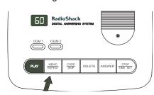
2. The TAD automatically stops recording after 60 seconds or you can press STOP/TIME SET when you finish the memo. The TAD beeps once, and the message number indicator increases by one.
