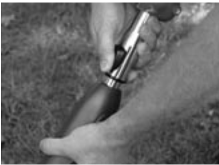
Figure 4-27: Sliding telescoping release button upward
