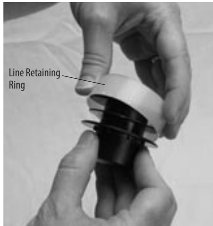
Figure 4-16: Removing line retaining ring
