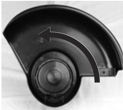
Figure 3-2: Rotating cutting guard into place
