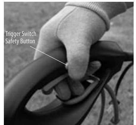
Figure 4-9: Pressing trigger switch safety button
