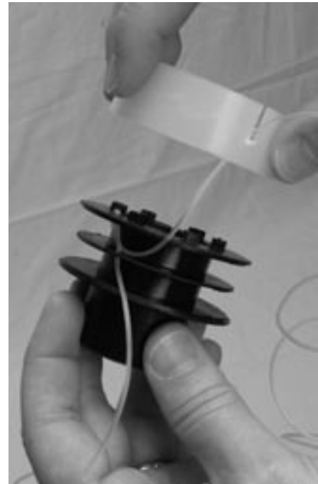
Figure 4-22: Placing retaining ring onto spool
