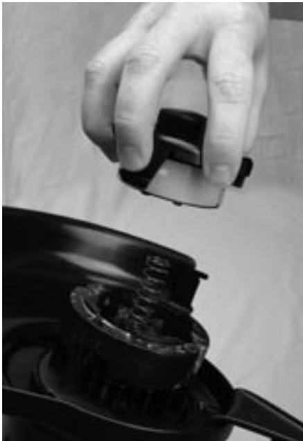
Figure 4-14: Removing spool cover and spool
