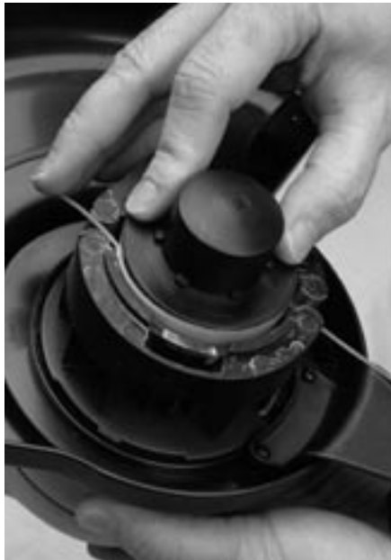
Figure 4-25: Replacing spool into spool housing
