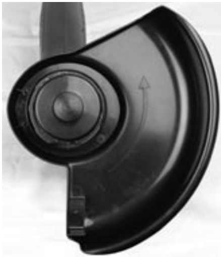
Figure 3-1: Placing cutting guard over cutting head
