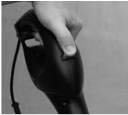
Figure 4-29: Pressing shaft rotation release button
