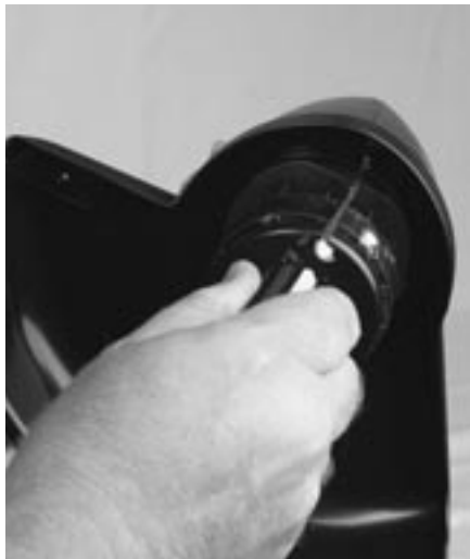
Figure 3-3: Attaching mounting screw
