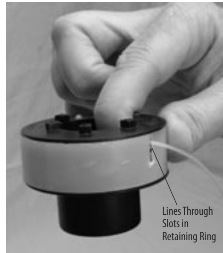
Figure 4-23: Positioning line in retaining ring slots
