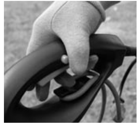
Figure 4-8: Holding trimmer/edger rear handle
