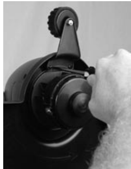
Figure 3-5: Attaching edging wheel
