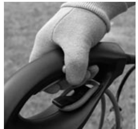
Figure 4-10: Squeezing trigger switch
