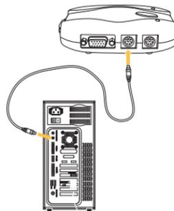
2. Connect one end of the PS/2 keyboard KVM cable to the keyboard port on the computer and the other end to the KEYBOARD 1 port on the side of the Switch.
