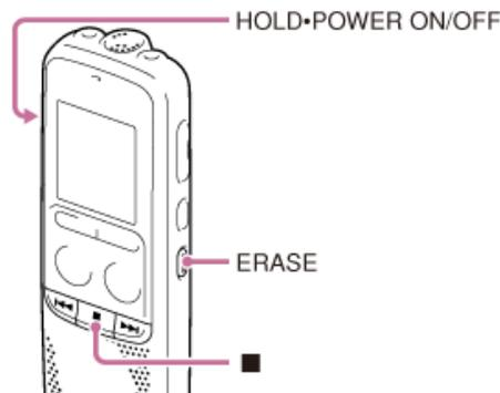
1. Slide the HOLD · POWER ON/OFF switch in the direction of "POWER ON/OFF" to turn on the IC recorder, or towards the center to release the IC recorder from the HOLD status.
