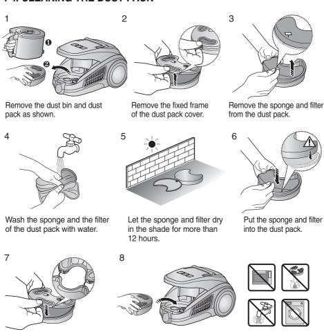
NOTE: Make sure the filter is completely dry before putting it back into the vacuum
