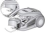
Pull out the HEPA Filter as shown.
