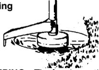
**SWEEPING** - The fanning action of the rotating line can be used for a quick and easy clean up. Keep the line parallel to and above the surfaces being swept and move the tool from side to side.
