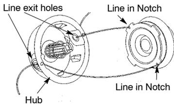
5. Wind the line evenly and tightly onto the spool. Wind in the direction of the arrows found on the spool.
