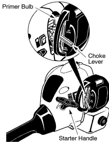
5. Pull starter rope handle sharply until engine sounds as if it is trying to start, but do not pull rope more than 6 times.
