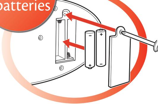
Use a Phillips/cross head screwdriver (not included) to loosen screw in battery compartment door (screw remains attached to door). Remove door. Remove old batteries. Insert 2 "AA" or R6 size batteries. Alkaline batteries recommended. Replace door and tighten screw.
