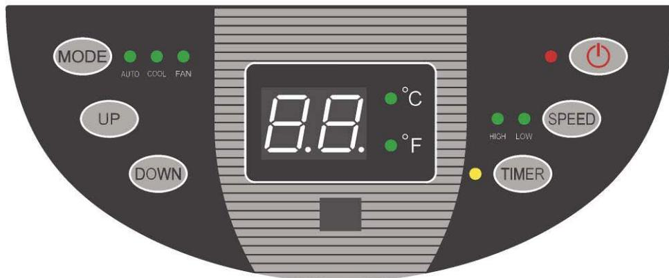
1. POWER button: press this button to turn on/off the unit.
