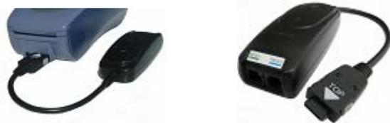
LinkBox provides a back-up dial connection (asynchronous and synchronous, V22bis or V34) and powered RS-232 port. ComBox provides two RS-232 ports, one of them powered (port marked RS232-2 provides power for the attached device).
