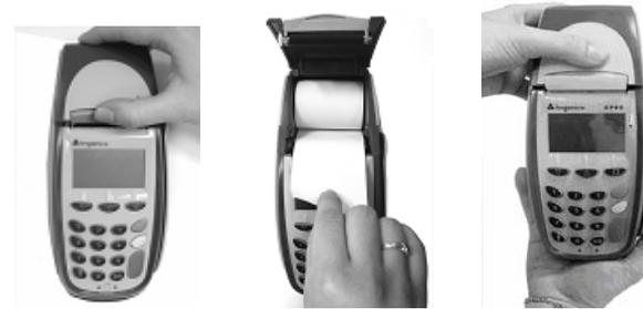
3. Close the cover, press it until it snaps. Power up the unit and press the blue "Paper feed" key to verify that paper feeds properly.
