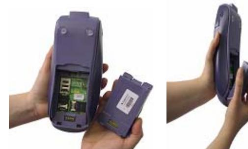
Insert the two plastic teeth in the gaps on the i7910 case, place the battery into the cavity and push it. Press the battery handle until a click is heard.
