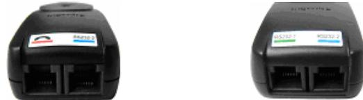
Connect LinkBox or ComBox to the i7910 RS-232 port, the letters "TOP" on a connector must be facing up. The green light (LinkBox only) indicates modem is ready. The light becomes red while dial connection is used.
