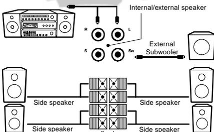
If you have connected external side speakers to the television, set the internal/external selection button (located at the rear of the television set close to the connectors) to the external position (pushed down). Use the point of a pen.
