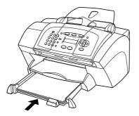
**6** To prevent paper from possibly falling off the tray, fully extend the output-tray extender.
