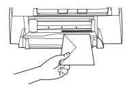
• If you are printing multiple envelopes, remove all paper from the input tray, and then slide a stack of envelopes into the tray, with the envelope flaps up and to the left (print-side down), until they stop.
