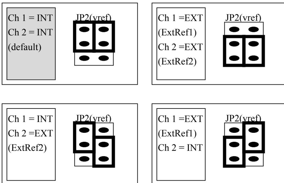
If JP2 is set to **internal reference**, then JP1 should be set to **-5V or -10V** internal reference voltage.
