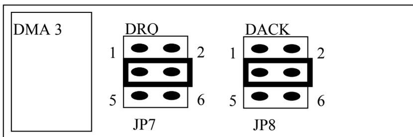
**The DMA channel can not shared.** The OME-A-822 software driver can support 8 different boards in one PC based system, but only **two of these boards** can use the DMA transfer function.
