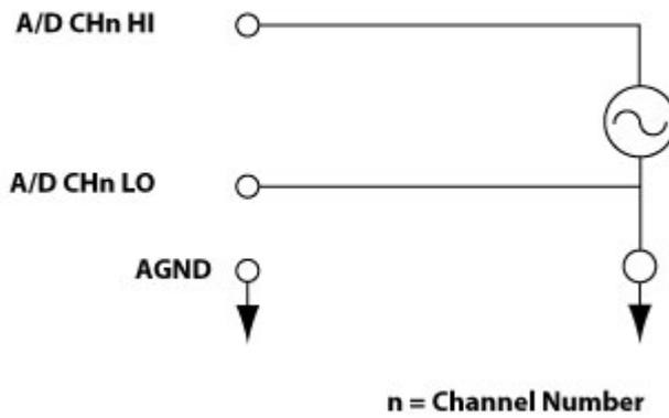
*If the source is grounded, a second ground connection on the card could result in a ground loop.*
