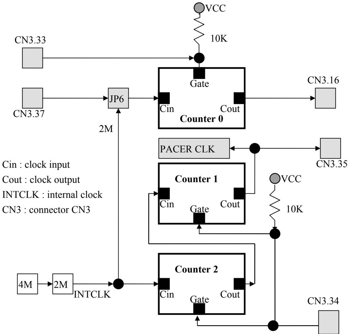
The counter0, counter1 and counter2 are all 16 bit counters. Counter 1 and counter 2 are cascaded as a 32 bit timer. This 32 bit timer is used as a **pacemaker timer**. The software driver, **A-822\_Delay()**, uses counter 0 to implement a machine independent timer for settling time delay (sec. 2.4.6 and sec. 2.4.7). If A-822\_Delay() is not used, counter0 can be used as a general purpose timer/counter.
