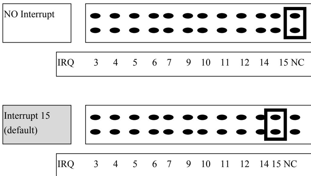
The interrupt channel **can not be shared**. The OME-A-822 software driver can support 8 different cards in one system but only **2 of these cards** can use the interrupt transfer function.
