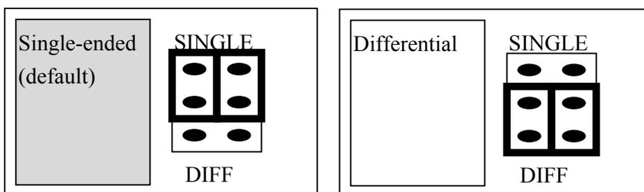
The OME-A-822PGL/PGH offers 16 single-ended or 8 differential analog input channels. The JP3 jumper sets the inputs to single-ended or differential mode. You can not select single-ended and differential simultaneously.
