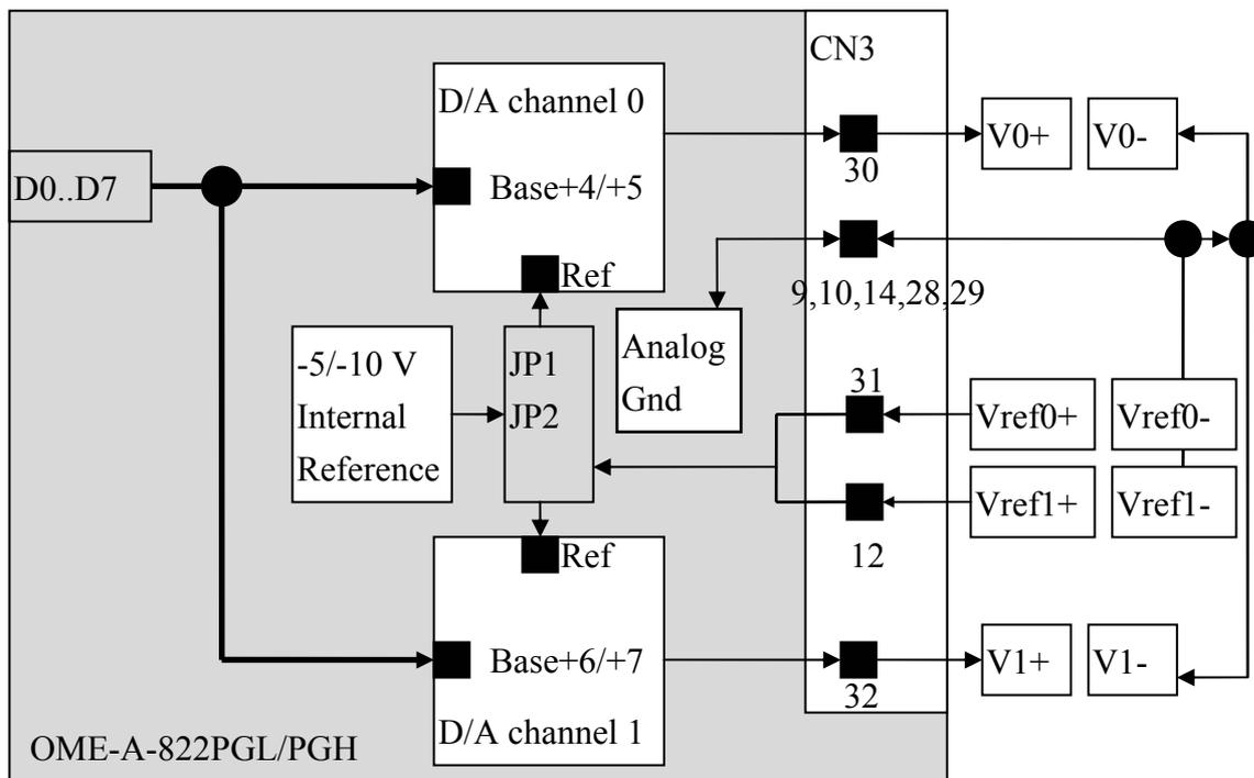
NOTE : The D/A output latch registers use a “double buffer” structure. **The user must send the low byte data first, then send the high byte data.** If the user only sends the high byte, the low byte data will be the previous value.
