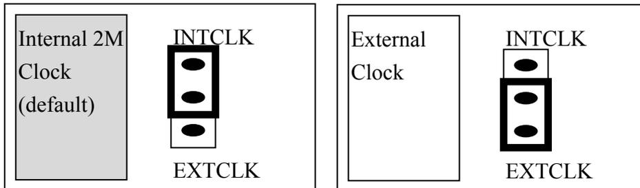
The OME-A-822PGL/PGH has 3 independent 16 bit timer/counters. The cascaded counter1 and counter2 are used as a **pacemaker timer**. Counter0 can be used as a user programmable timer/counter. The user programmable timer/counter can be set to **2M internal clock** or **external clock ExtCLK, CN3 pin 37**. The block diagram is given in section 2.6. The clock source must be very **stable**. Using the 2M internal clock is strongly suggested.
