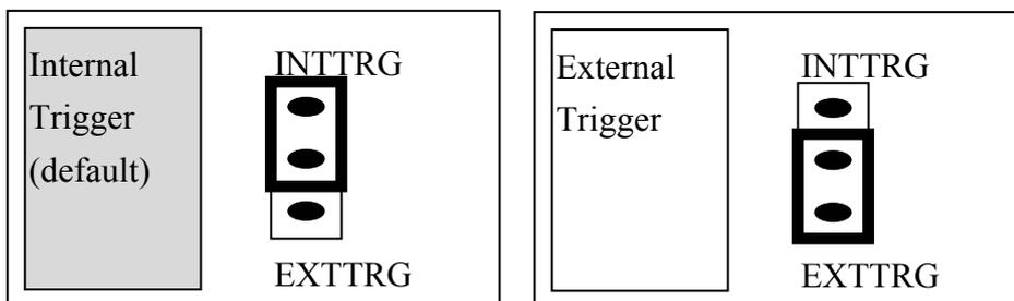
The OME-A-822PGL/PGH supports two trigger types, **internal trigger** and **external trigger**. The external trigger comes from **ExtTrg, CN3 pin 17**. There are two types of internal triggers, **software trigger** and **pacer trigger**. More detailed information is given in section 2.4.8.
