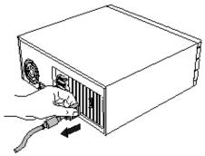
**Note:** If you are disconnecting a peripheral from the computer or are removing a component from the system board, wait 10 - 20 seconds after disconnecting the computer from the electrical outlet before disconnecting the peripheral or removing the component to avoid possible damage to the system board. To verify that all power has been removed from the system, make sure that the standby power light-emitting diode (LED) on the system board has gone out.
