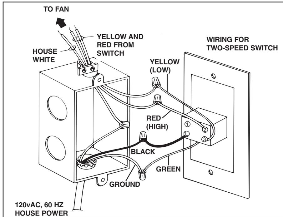
1. Switch installs in single-gang outlet box.
