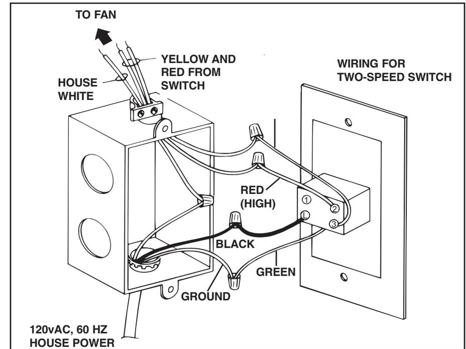
1. Switch installs in single-gang outlet box.
