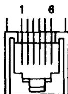
Connector used : TM5RJ3-66 (Hirose) or equivalent
