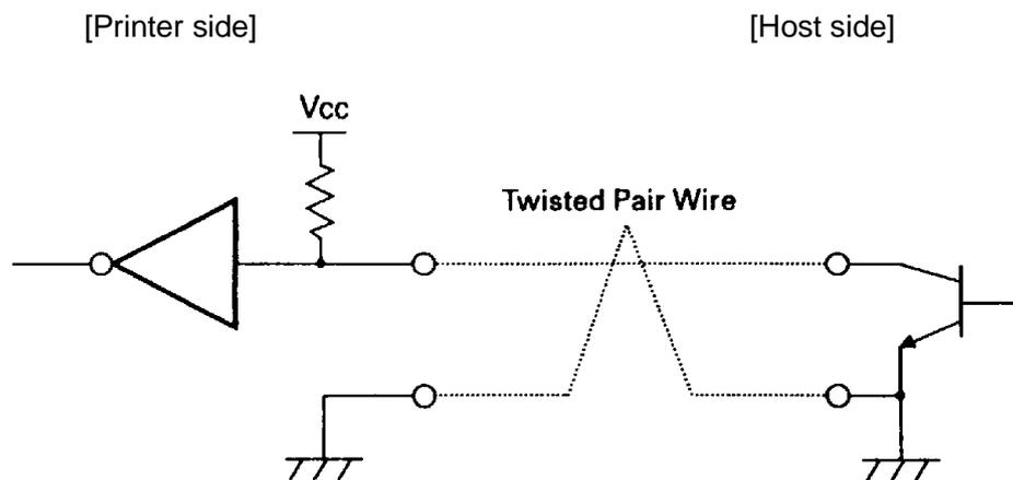
All the output signals are pulled up by 50K $\Omega$ .
